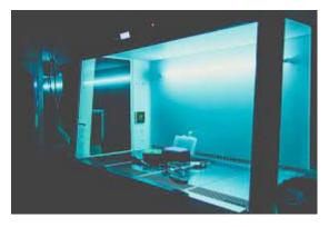
These are used for sterilization and disinfection, although their use for these purposes is no longer recommended. If you have questions about alternate methods of sterilization and disinfection, please reach out the Biosafety Office.
