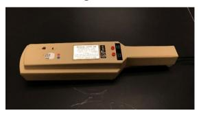
These are used primarily for visualizing nucleic acids following staining.
