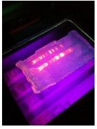
These are used for the visualization of DNA following gel electrophoresis and ethidium bromide staining.
