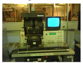
These are used to transcribe a fine pattern on a substrate using UV light. Substrates are made of various materials like silicon, glass, ceramic, GaAs, quartz, etc. They are used in the manufacturing of semiconductor devices, such as general transistors and Integrated circuits, and also used for LCD glass patterns and quartz crystal units.ii
