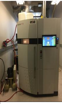
EOS Formiga P110 Laser Sintering 3D printer (Industrial-grade)
