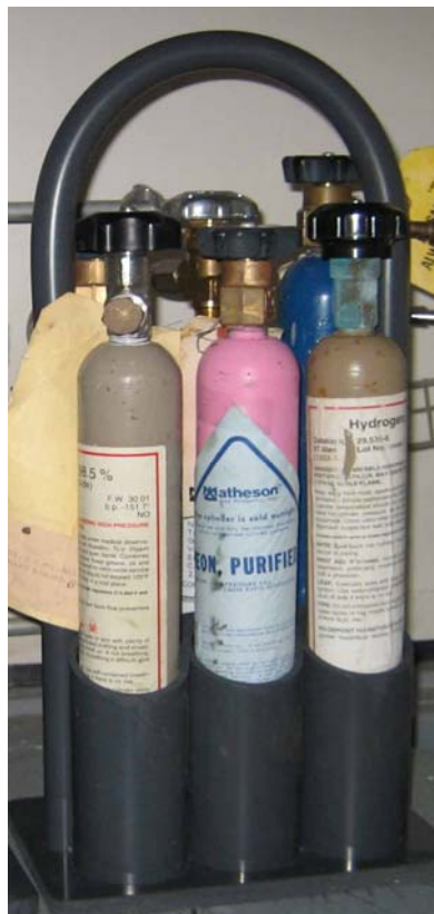
Holder available from Sigma appropriate for storing lecture bottles
